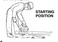
WARNING: When starting engine, hold the unit as illustrated. Do not set unit on any surface except a clean, hard area when starting engine or while engine is running. Debris such as gravel, sand, dust, grass, etc. could be picked up by the air intake and thrown out through the discharge opening,
